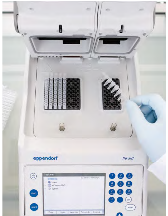
Run two separate PCRs at the same time with Mastercycler® nexus X2
